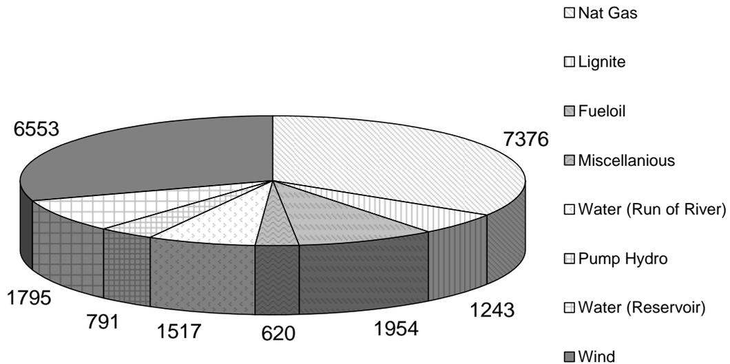
Fig. 1.4. Installed power plant capacities base case in 2030
