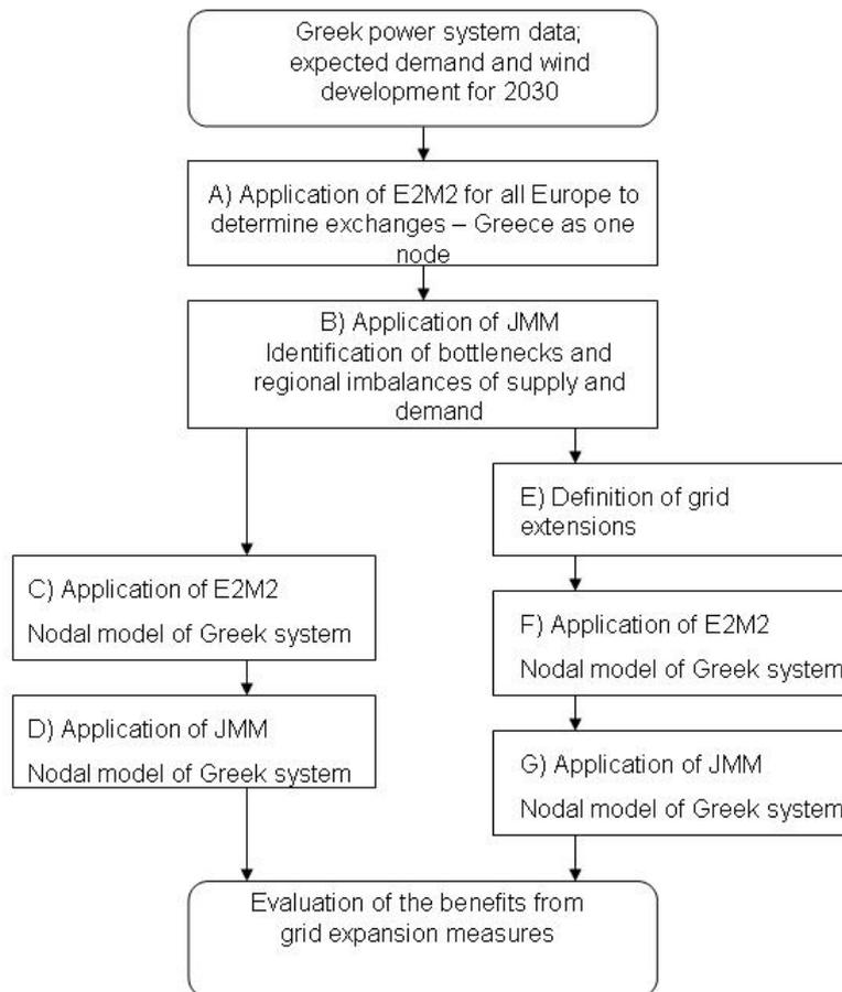
Fig. 1.1. Sequence of model runs performed
